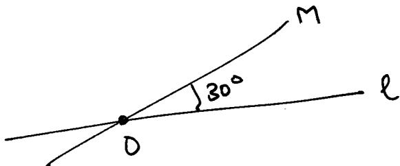
$M \circ \ell =$  counter clockwise rotation about  $O$  through  $2(30) = 60^\circ$ .
