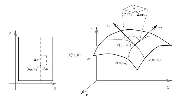
The parametric map  $\mathbf{r}(u, v)$  takes a rectangle of side lengths  $\Delta u$  and  $\Delta v$  to a curvilinear patch on the parametric surface in 3-d as shown in the diagram. The area of this patch is approximated (up to first order) by the area of a parallelogram in 3-d with sides given by the tangent vectors  $\Delta u \mathbf{r}_u$  and  $\Delta v \mathbf{r}_v$ . This area is just
